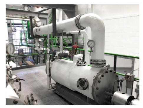
We have 5 distillation units, but out largest production unit is an all stainless steel, two column, continuous still. The feed rate is up to 500 lbs/hr for dry vacuum distillation.
